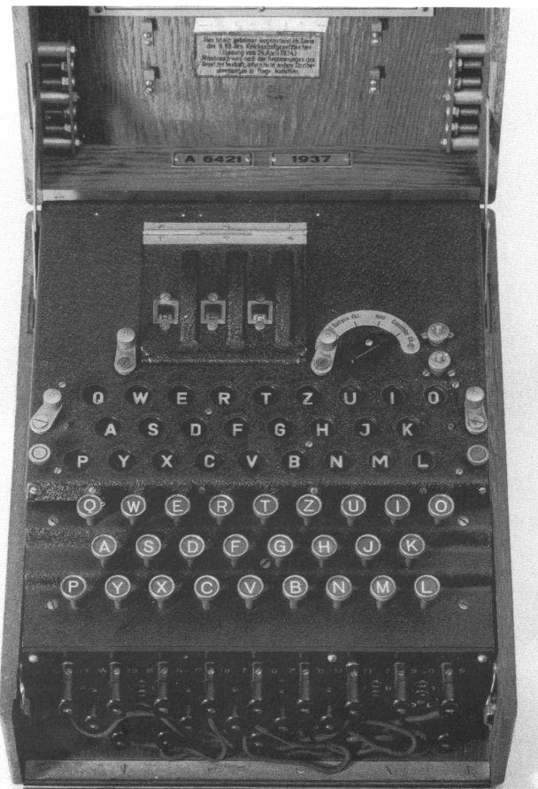
2. Typical 3-wheel Army Enigma, with inner lid closed, showing the 3-letter setting; note the warning about secrecy
